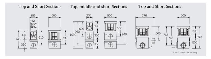
Multipart construction with multiple combination possibilities of upper, middle and lower gully. Includes integrated stainless steel edge protection. Sediment buckets made from galvanised steel also available. Suitable with above stainless steel grates with standard locking mechanisms. Includes preformed outlet knockouts making the perfection connection for LS/Z2000.0, Z/S2010.0 and Z/S2020.0 channels.
